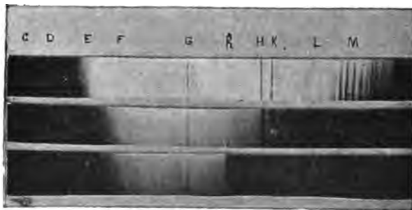
FIG. 43.— Photographs showing the disappearance of the solar ultra-violet on certain days caused by unknown influences. —The upper band represents an ordinary solar spectrum extending to the borders of the N ray. The band beneath it shows the disappearance of the solar ultra-violet starting from the L ray, notwithstanding the prolongation of the exposure. The lower band represents the total disappearance of the ultra-violet when the spectrum is photographed through a transparent solution of sulphate of quinine.
